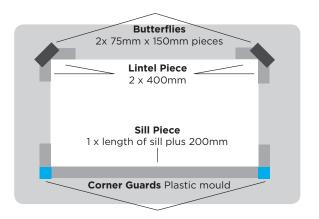
Apply Masons Hydro Flashing Tape to top of window head flashing, upstand and building wrap. Refer to window & cladding details for specific application.
